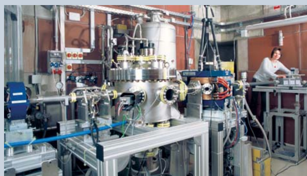
Fig. 2: Beamline of the channeling X-ray facility at ELBE. The electron beam coming from the ELBE accelerator (from the left) and entering the vacuum chamber (in the middle) hits a single diamond crystal. Channeling radiation is emitted by the relativistic electrons when traveling through the crystal along a lattice plane.
