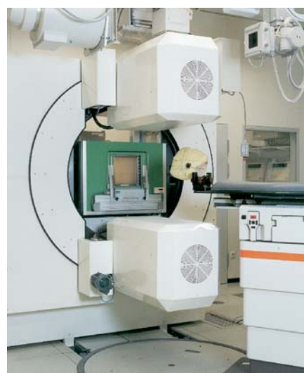
Fig. 1: Double head positron camera developed by FZD at the treatment site of GSI Darmstadt. The horizontal carbon ion beam leaves the beam pipe through a 20 x 20 cm 2 window visible in the centre of the picture. To provide sufficient space for patient positioning, the PET scanner can be moved on rails parallel to the beam between the measuring position displayed and the parking position upbeam. (Photos: GSI)
