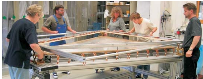
Fig. 2: Mounting and testing one of the six multi-wire chambers in the detector workshop at the FZD. The six chambers are arranged hexagonally, forming a large frustum around the beam direction. Their position is colored red in Fig. 1.
