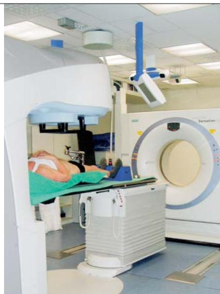
**Fig. 6:** The medical electron linear accelerator Oncor Impression (Siemens Health Care) – left – equipped with gating beam delivery technology and an in-room X-ray computer tomograph – right – for image guided adaptive radiotherapy at the University Hospital Carl Gustav Carus, Dresden.
