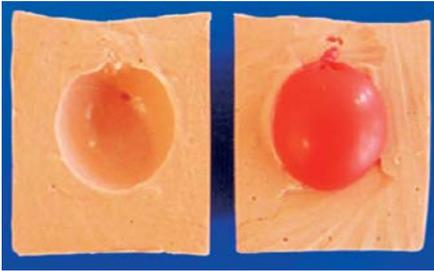
**Fig. 3:** Balloon phantom filled with a water/ethanol (5%) mixture and embedded in an alginate molding.
