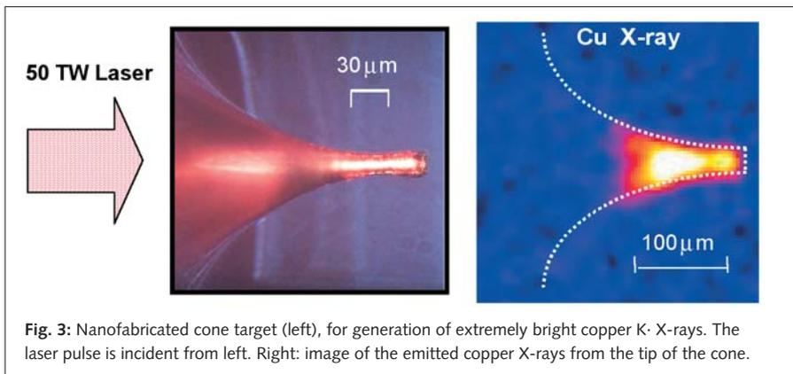
**Fig. 3:** Nanofabricated cone target (left), for generation of extremely bright copper K- X-rays. The laser pulse is incident from left. Right: image of the emitted copper X-rays from the tip of the cone.
