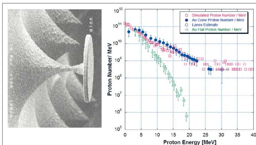
**Fig. 1:** Electron microscope picture of a nanofabricated laser-proton acceleration target made from 10  $\mu\text{m}$  thick gold (left). The high intensity laser is incident from the left into the interior of the cone; protons are accelerated from a hydrogen layer on the flat disk. The spectrum of accelerated proton energies (right) exhibits a 4-fold greater flux and higher energy range (blue data) as compared to a flat foil target (green points).
