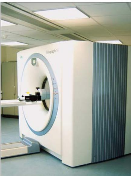
**Fig. 5:** The PET/CT scanner Biograph 16 (Siemens Health Care) equipped with 4D imaging capability at the University Hospital Carl Gustav Carus, Dresden.
