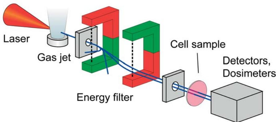
**Fig. 1:** Experimental setup at the JeTi laser electron accelerator: The laser pulses are focused into a helium gas jet, ionizing the gas and generating a plasma wave. Electrons are accelerated and filtered by permanent magnets and collimators. Behind the filter, a homogeneous electron beam passes through the cell sample and is detected by several detectors and dosimeters.
