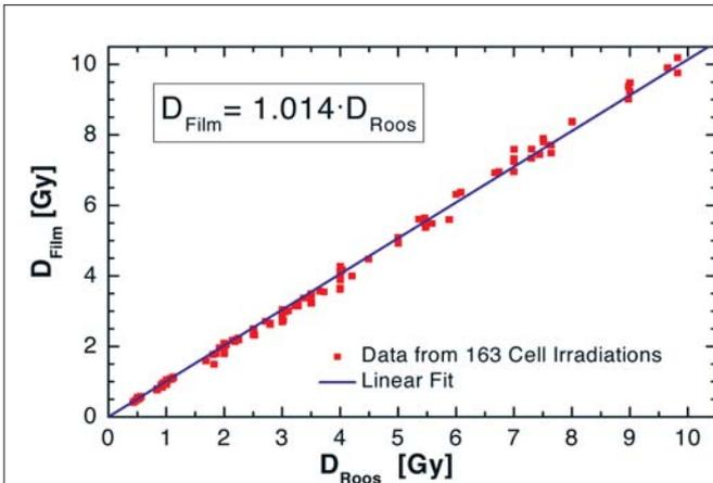
**Fig. 3:** Correlation of the doses measured online with a Roos ionization chamber and retrospective with EBT radiochromic films for the irradiation of 163 cell samples over two months.
