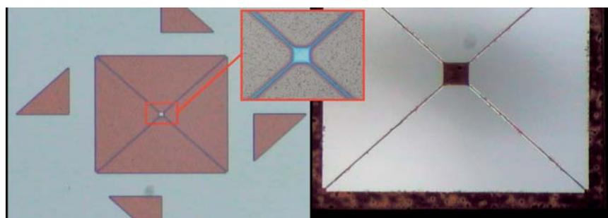
**Fig. 2:** Next generation of reduced mass targets, produced by semiconductor processing techniques in the Ion Beam Center. Left: Silicon wafer mounting structure (0.5 mm x 0.5 mm open area), with 10  $\mu\text{m}$  x 10  $\mu\text{m}$  target (inset), during fabrication. The triangles are fiducial marks to aid in the laser beam alignment. Right: completed free-standing 50  $\mu\text{m}$  x 50  $\mu\text{m}$  target.
