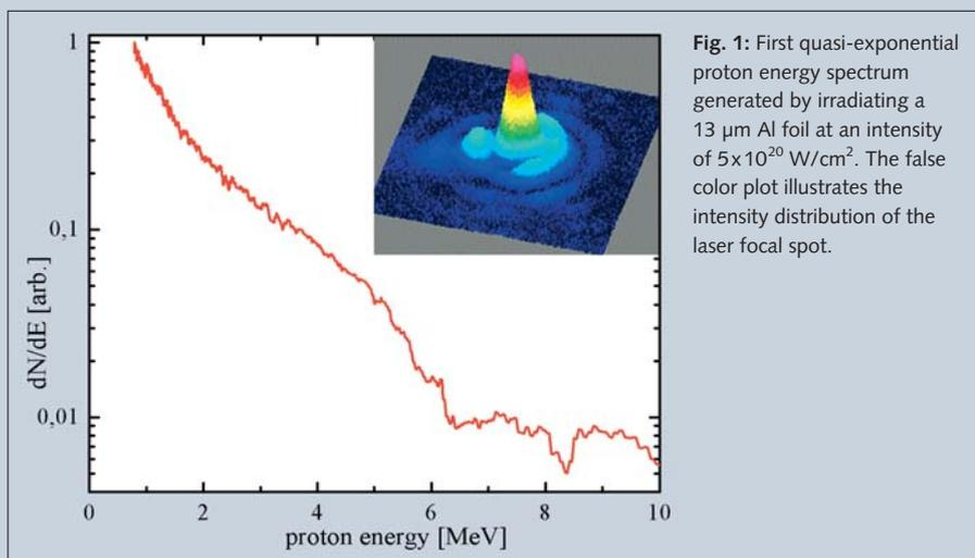
**Fig. 1:** First quasi-exponential proton energy spectrum generated by irradiating a 13  $\mu\text{m}$  Al foil at an intensity of  $5 \times 10^{20} \text{ W/cm}^2$ . The false color plot illustrates the intensity distribution of the laser focal spot.
