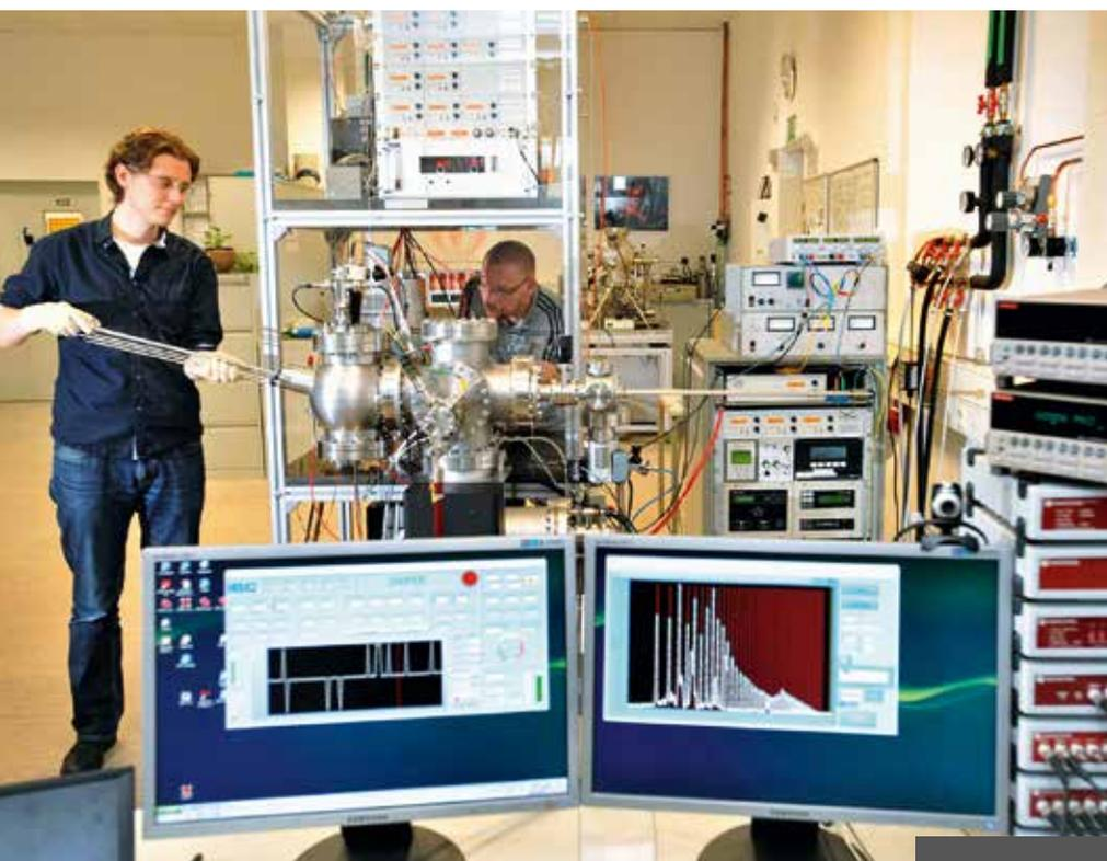
**NANO-STRUCTURES:** This facility will make it possible to implant individual ions into a surface of mere square nanometers like precision projectiles. Richard Wilhelm (left) and René Heller calibrating the ion beam. Photo: Frank Bierstedt
