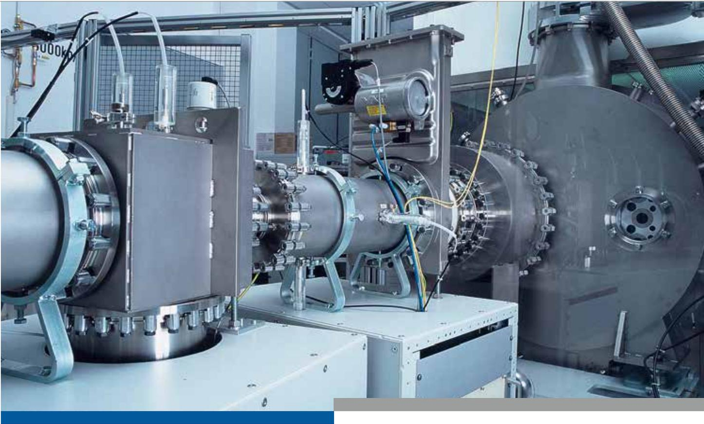
**ION MACHINE:** Low-energy ions knock atoms out of their normal positions in the crystal lattice. Photo: Claus Preußel
