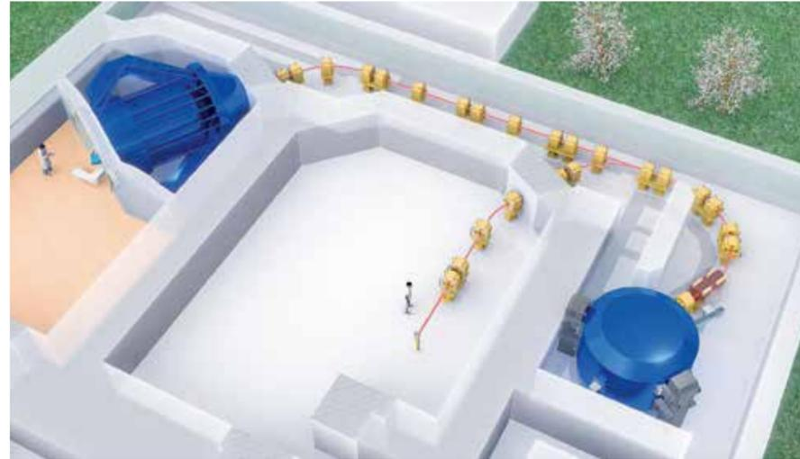
The construction in Dresden is one of a handful worldwide that allow patients to be treated in the gantry (left) and experiments with charged particles to be conducted in a special experimental space (middle). The protons are generated by the ring accelerator (right). Source: OncoRay
