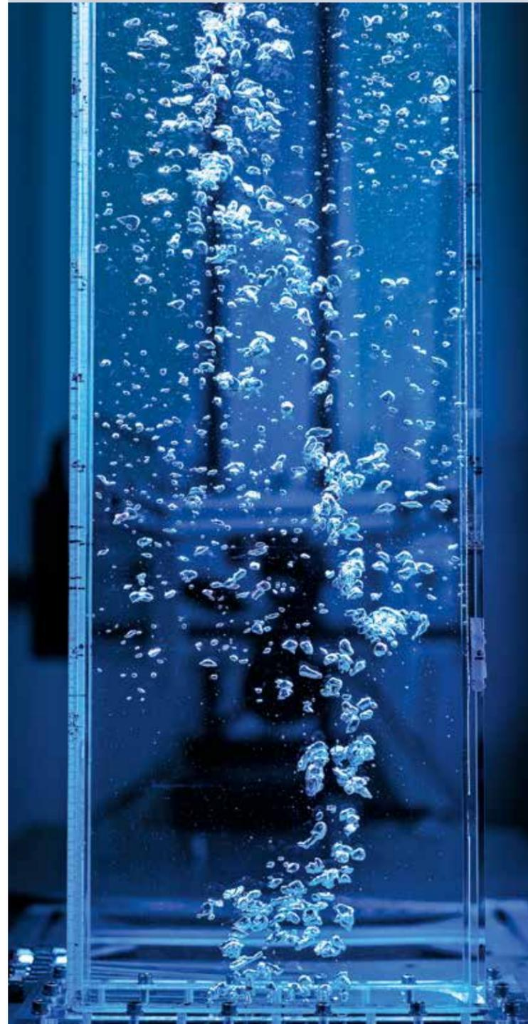
┘ Unlike the reactors used in the chemical industry, the flow processes can be easily observed in transparent bubble columns. The similarity between the processes in both set-ups allows researchers to precisely investigate flow conditions. Source: A. Wirsig ┘
