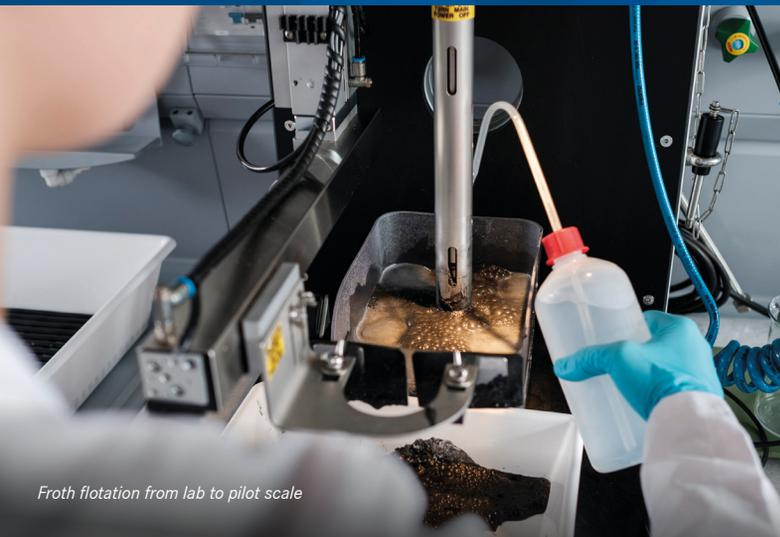
Froth flotation from lab to pilot scale
