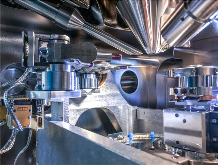
Figure 1: A set of four micromanipulators mounted on the He-FIB tilt stage
