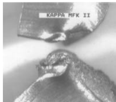
Fig. 2.21.. A side view on the final zone of fracture surface in a dynamic fracture toughness test. Note that the surface of the lower sample half practically follows the shape of striker tip. Sample H145, steel A508.
