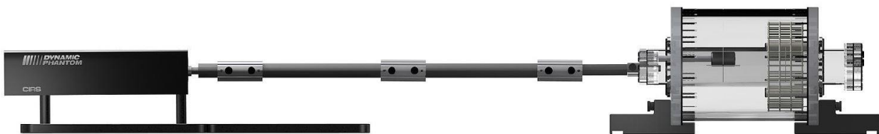
Fig. 1. Schematic setup of the MRI-LINAC Dynamic Phantom [12] comprising an actuator [left], modular extension shafts [middle], and movable cylinder with simulated target inserted into a torso-shaped body [right].
