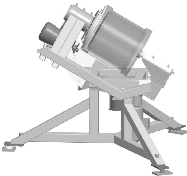
Figure 2. Sketch of the water experiment. Compared to the planned large scale experiment the water device is smaller by a factor of 6.
