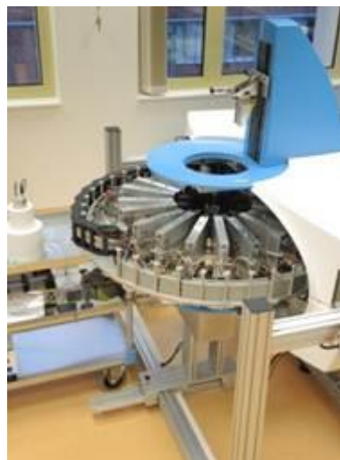
Fig. 2: Aligned axes of the sample and FOV by tilting of the complete scanner. The sample is fixed on a rotary table below the gantry.
