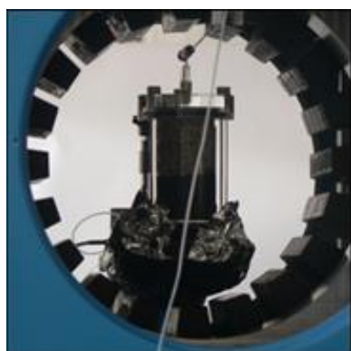
Fig. 1: Disadvantageous vertical orientation of the sample in the horizontally oriented FOV .
