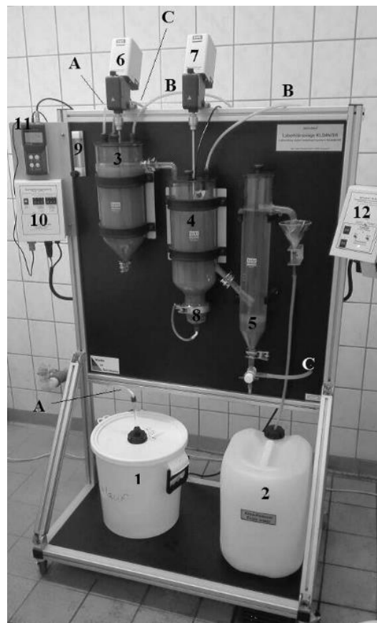
Fig. 1: Model waste water treatment plant KLD 4N/SR.: Supply of synthetic waste water (25 L) (1), cleared waste water (30 L) (2), denitrification reactor (3), nitrification reactor (4), clarifier (5), stirrers (6) & (7), aeration frit (8), oxygen flow regulation (9–11), return sludge regulation (12), inlet tube (A), internal recirculation (B), return sludge tube (C).
