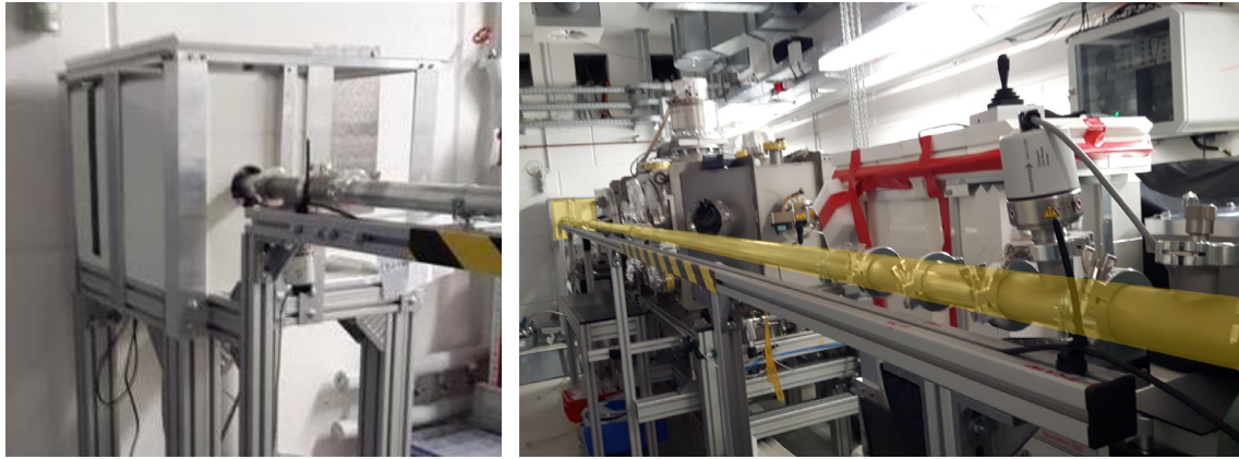
(a) Lead shielding of Pixis camera.
