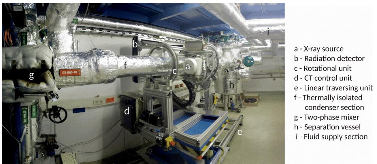
381 Figure 9: COSMEA facility at HZDR with the X-ray CT scanner.
