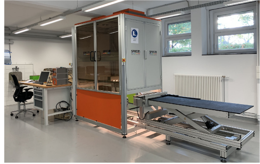
Fig. 3. SisuRock drill-core scanner equipped with an AisaFenix VNIR-SWIR HS sensor.
