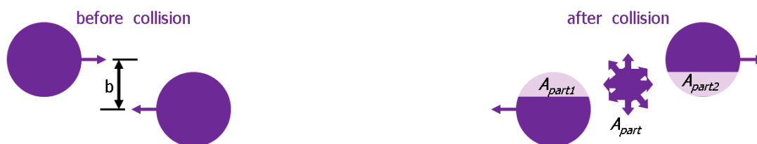
Figure B.1: A sketch of two nuclei before and after collision. The impact parameter quantifies the number of participants A_{part} affected in the geometrical overlap region of the reaction. The model allows prediction of the functional dependence of the number of participants on the impact parameter.
