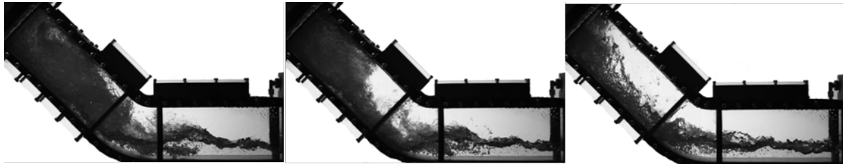
Fig. 1 Droplet formation at the wave crest (rolling wave flow condition at WENKA channel)
