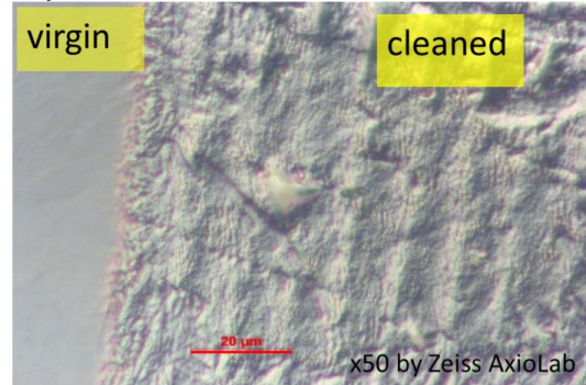
Figure 5: surface structure changes after cleaned with high intensity laser.
