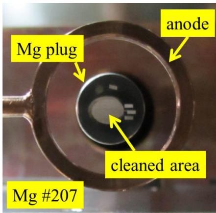
Figure 4: Photo of Mg photocathode #207 in transport chamber. This cathode has been cleaned for three times and used in gun twice for beam production.
