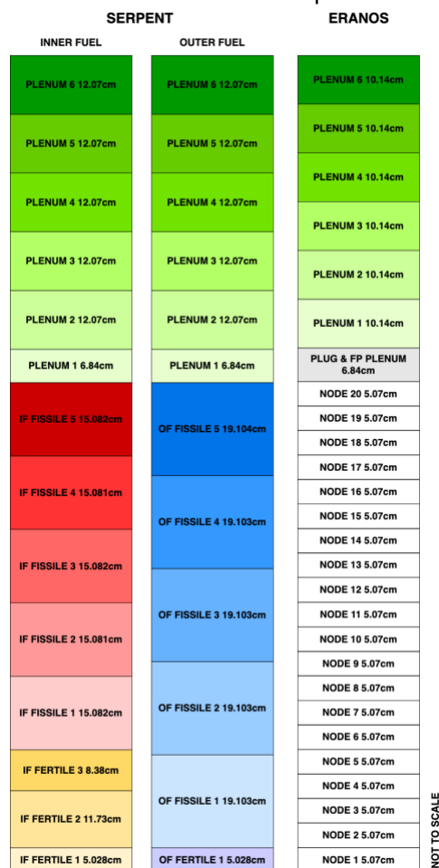
Figure 17 – Axial nodalisation of Serpent and ERANOS for sodium worth calculations
