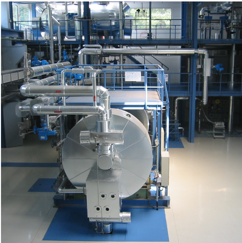
Fig. 2.7 View of TOPFLOW with the BWR emergency condenser test in the foreground
