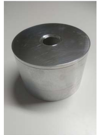
Figure 4.44: Aluminum sample holder for TU1. It consists of three distinct parts for different heights.
