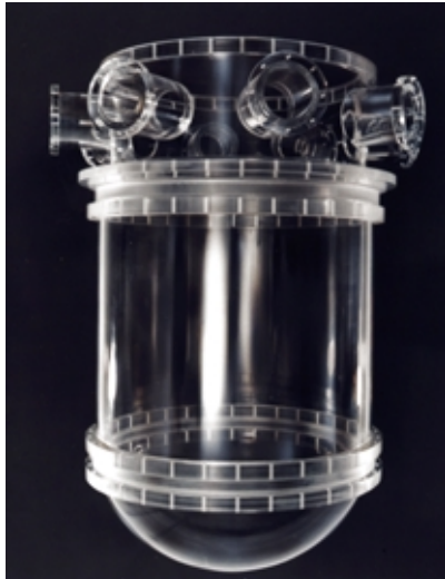
Fig. 2: RPV Plexiglas® Model
