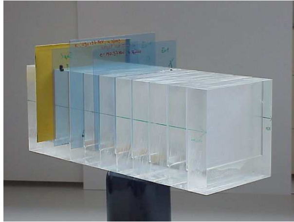
Figure 5–38: PMMA phantom with air gaps for insertion of radiographic emulsions.
