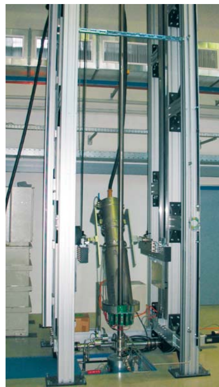
Fig. 2: ROFEX scanner at a vertical test section of the TOPFLOW facility.
