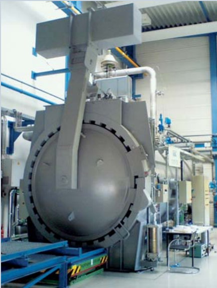
Fig. 2: TOPFLOW pressurized vessel for the operation of test sections and components in pressure equilibrium with the vessel atmosphere. This technology allows the application of optical and IR measurement techniques at pressures up to 50 bars.
