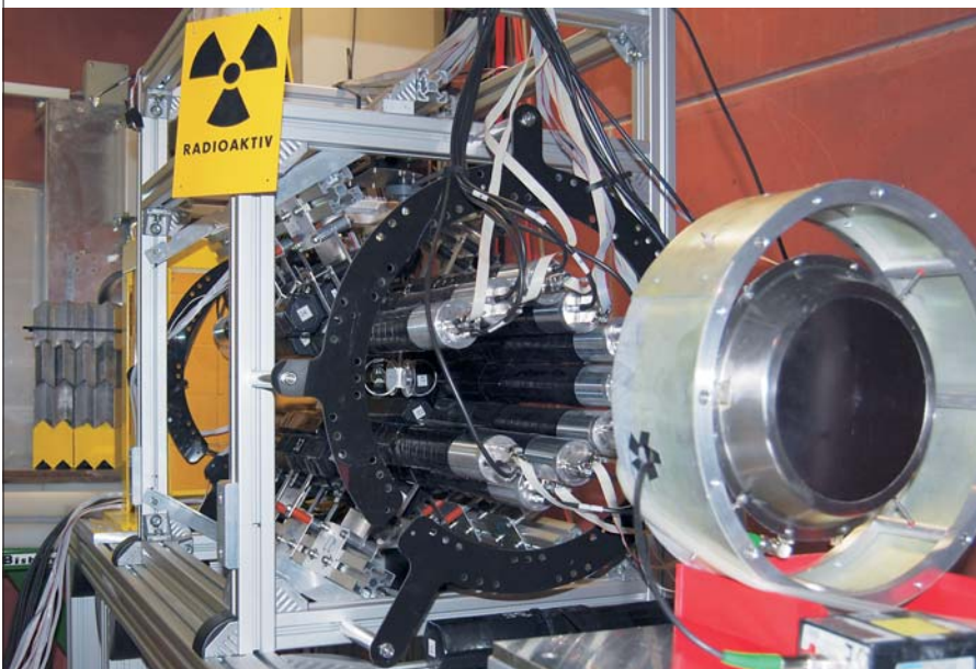
Fig. 3: The inelastic neutron scattering experiment from downstream direction. The neutron beam travels through the Barium-Fluoride ( \text{BaF}_2 ) detector array in the middle of the picture and passes the ^{235}\text{U} fission chamber from Physikalisch-Technische Bundesanstalt (PTB) on the right side, to be stopped in a beam dump. The target is located at the center of the \text{BaF}_2 array, for example a sample of ^{56}\text{Fe} , from which neutrons are scattered. Neutrons are detected by plastic scintillation counters on the left side (yellow). The simultaneously emitted photons are measured in the \text{BaF}_2 array.
