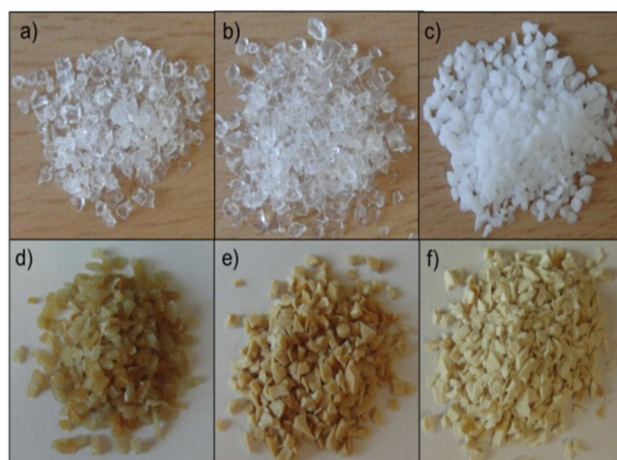
Fig. 1: Ceramics without (a-c) and with 20% biomass (d-f). Biocer 1(a & d), biocer 2 (b & e) and biocer 3 (c & f).
