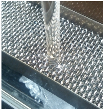
Figure 4.14: Strainer at the bottom of the window in series B
