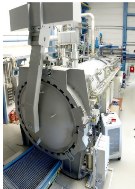
Figure 2.2: TOPFLOW pressure Tank B04
