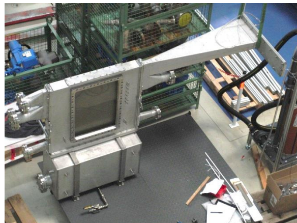
Figure 2.11: Basin B15 during the first tightness test.
