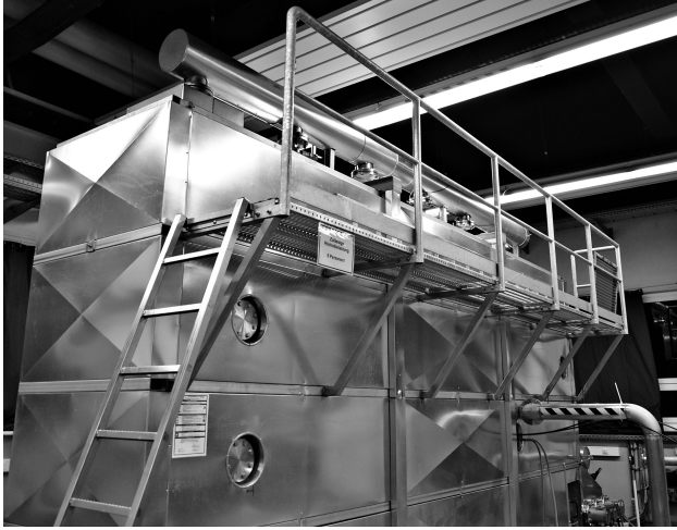
Figure 6: Test facility Zittau Flow Tray, a PWR scaled sump model with maximum capacity of 18\text{ m}^3
