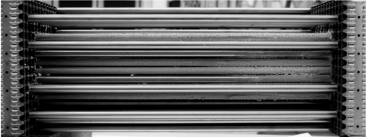
Figure 18: CP caused blockings inside the FA dummy (in dried state, after exp. no. ZFT-BE-V01; flow direction from left to right)
