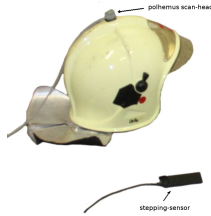
Figure 3: position sensor mounted to helmet
